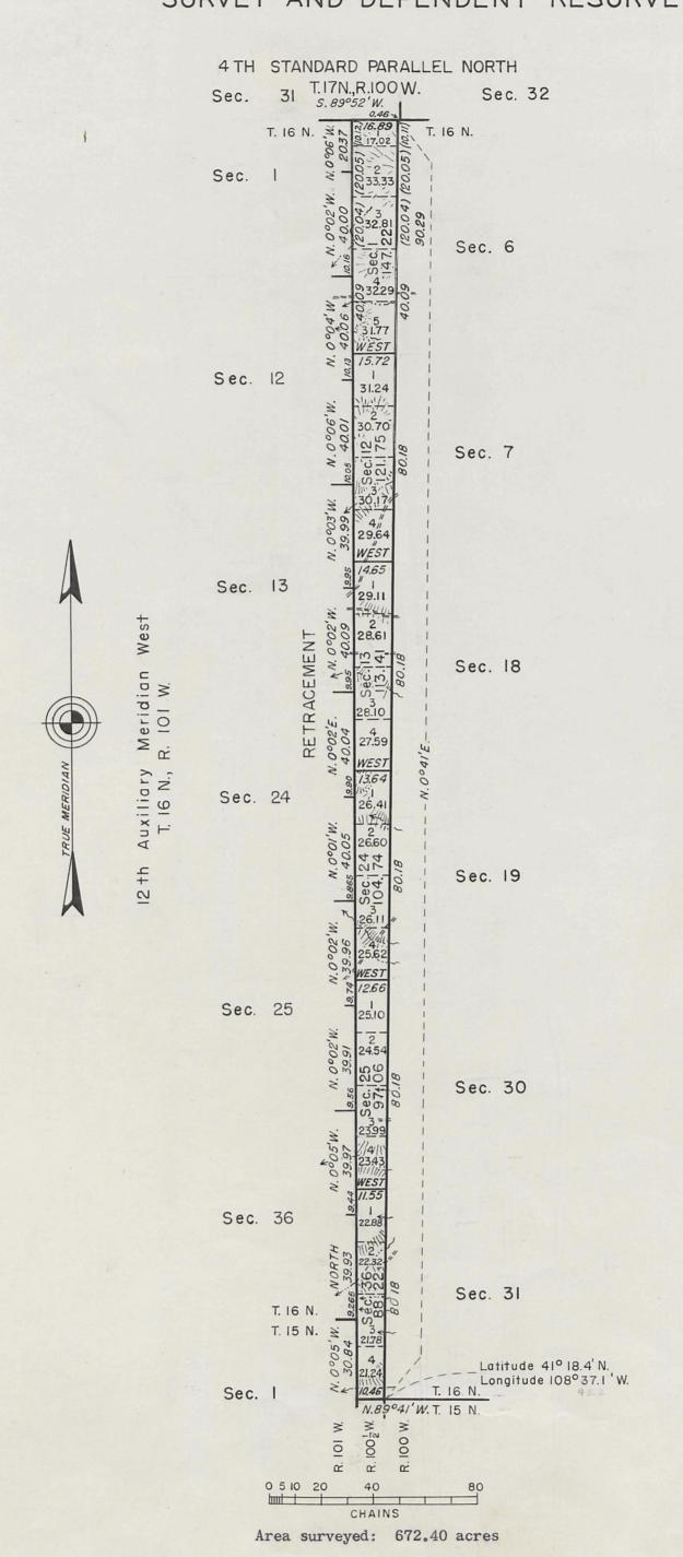
This plat represents a resurvey of the West boundary of T. 16 N., R. 100 W., and the East boundary of T. 16 N., R. 101 W., designed to restore the corners in their original locations according to the best available evidence, and a survey of the subdivisional lines of T. 16 N., R. 100½ W.
