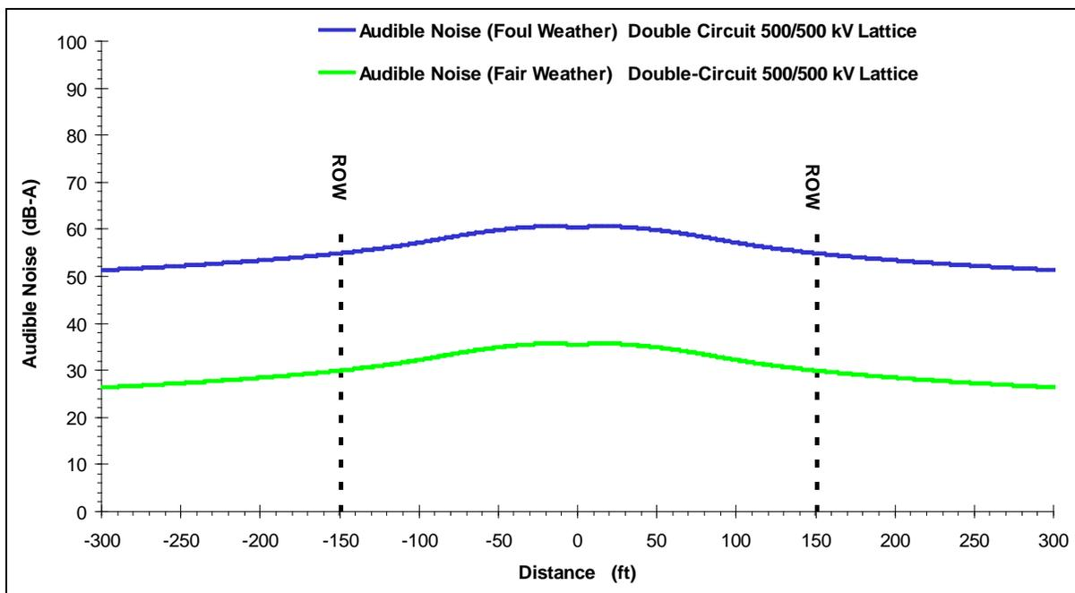
**Figure 3.21-13.** Audible Noise Profile at Midspan for Double-Circuit 500-kV Lattice Structure with Two 500-kV Circuits
