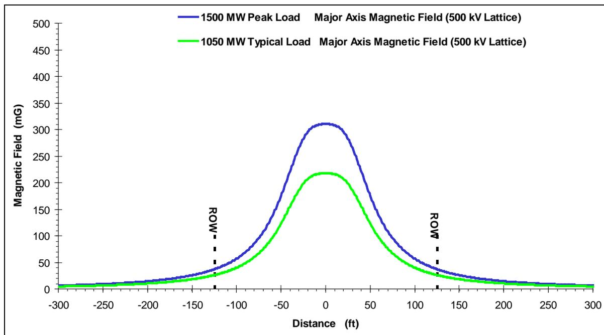
**Figure 3.21-8.** Magnetic Field Profile at Midspan for 500-kV Lattice Structure
