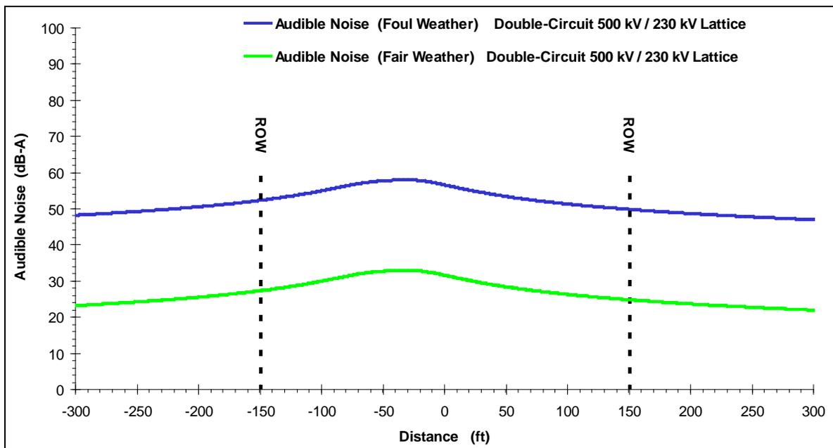
**Figure 3.21-14.** Audible Noise Profile at Midspan for Double-Circuit 500-kV Lattice Structure with a 500-kV Circuit and a 230-kV Circuit
