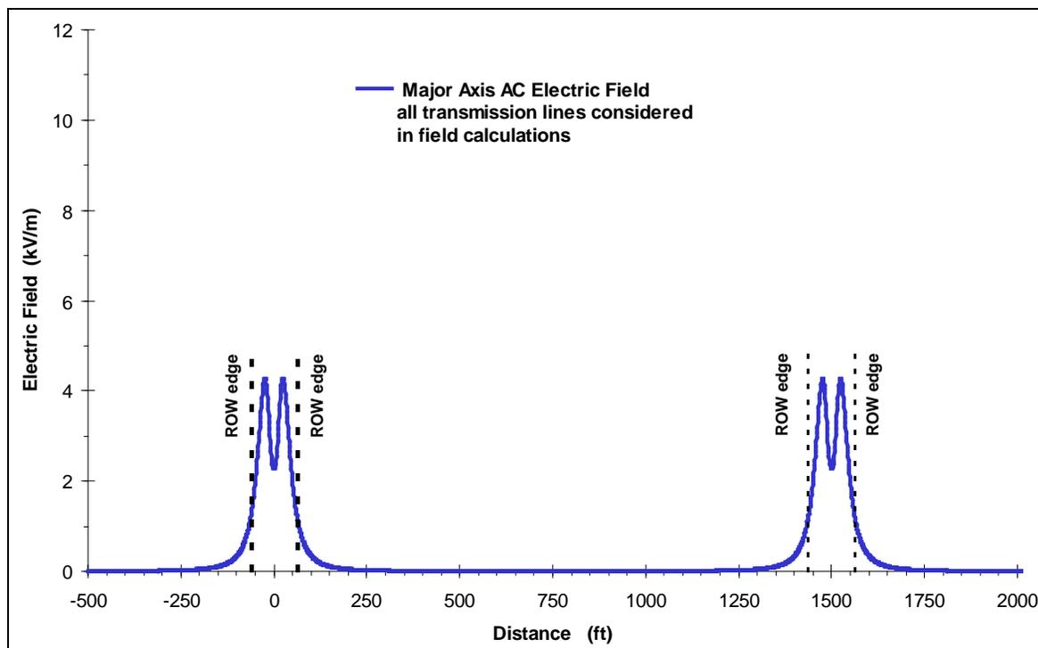
**Figure 3.21-1.** Plot of the Electric Field for Segment 1W Considering Two Parallel Lines 1W(a) and 1W(c) Separated from Each Other by 1,500 Feet in the Electric Field Calculations
