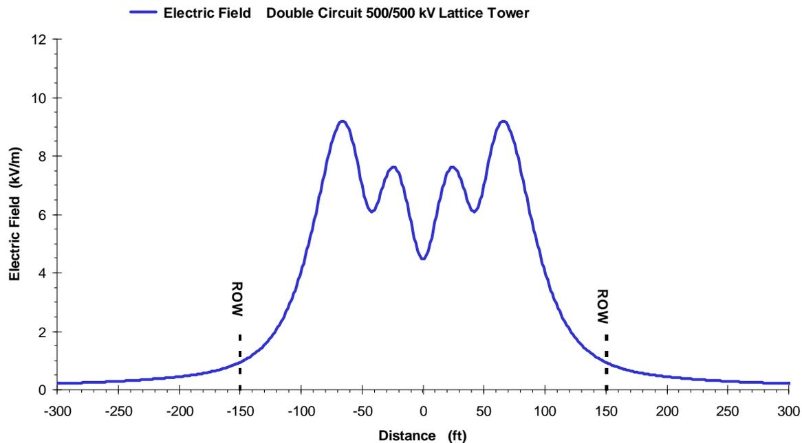
**Figure 3.21-5.** Electric Field Profile at Midspan for Double-Circuit 500-kV Lattice Structure with two 500-kV Circuits
