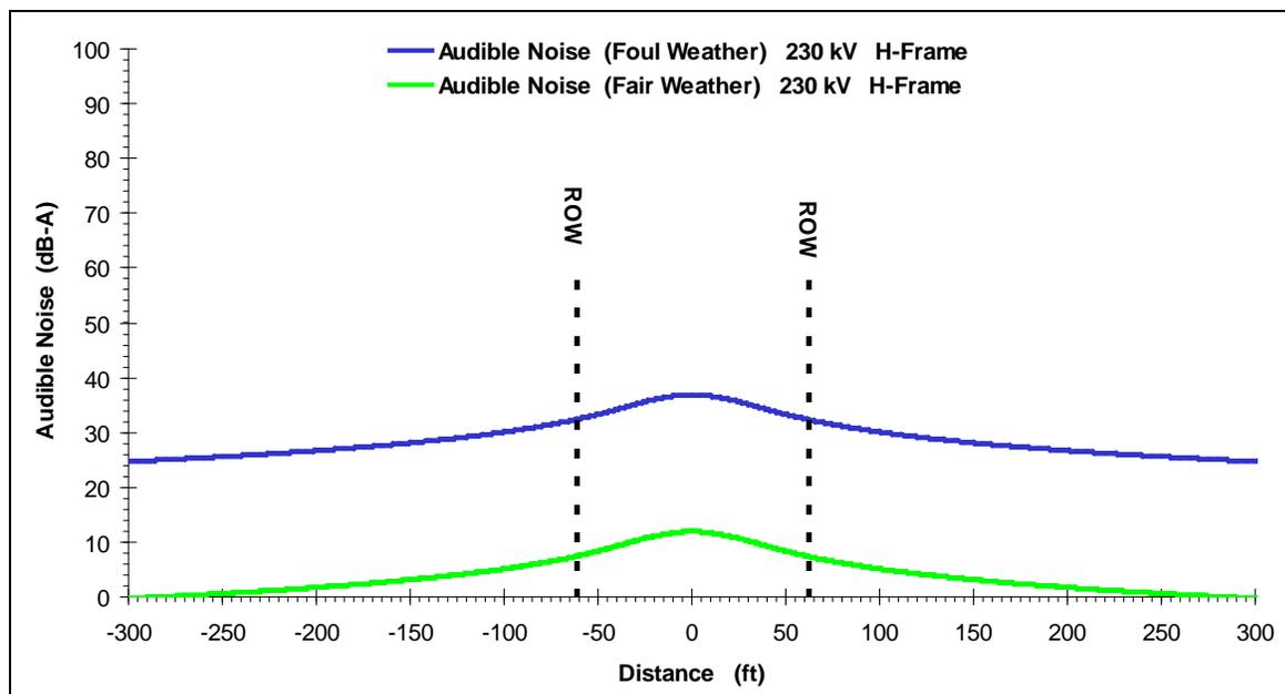
**Figure 3.21-11.** Audible Noise Profile at Midspan for Single-Circuit 230-kV H-frame Structure
