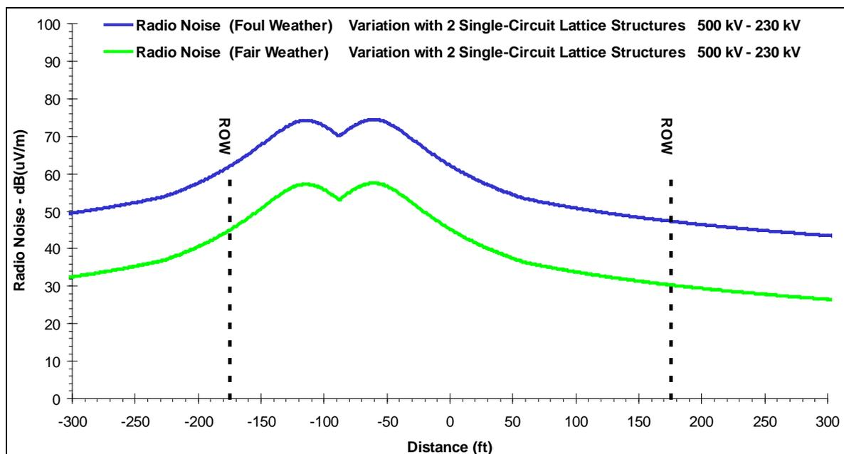
**Figure 3.21-27.** Radio Noise Profile at Midspan for Two Single-Circuit 500-kV Lattice Structures
