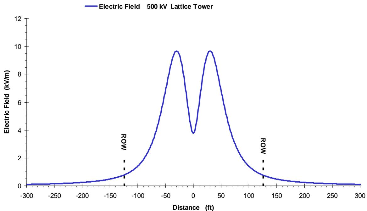
**Figure 3.21-4.** Electric Field Profile at Midspan for Single-Circuit 500-kV Lattice Structure
