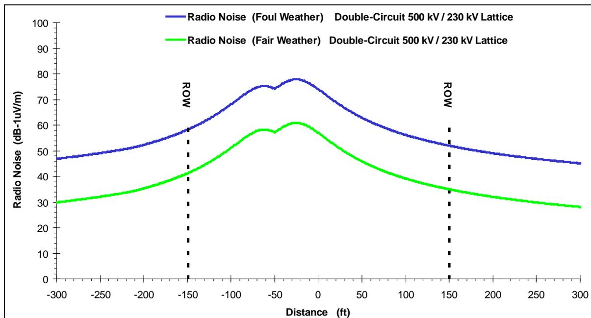
**Figure 3.21-18.** Radio Noise Profile at Midspan for Double-Circuit 500-kV Lattice Structure with a 500-kV Circuit and a 230-kV Circuit
