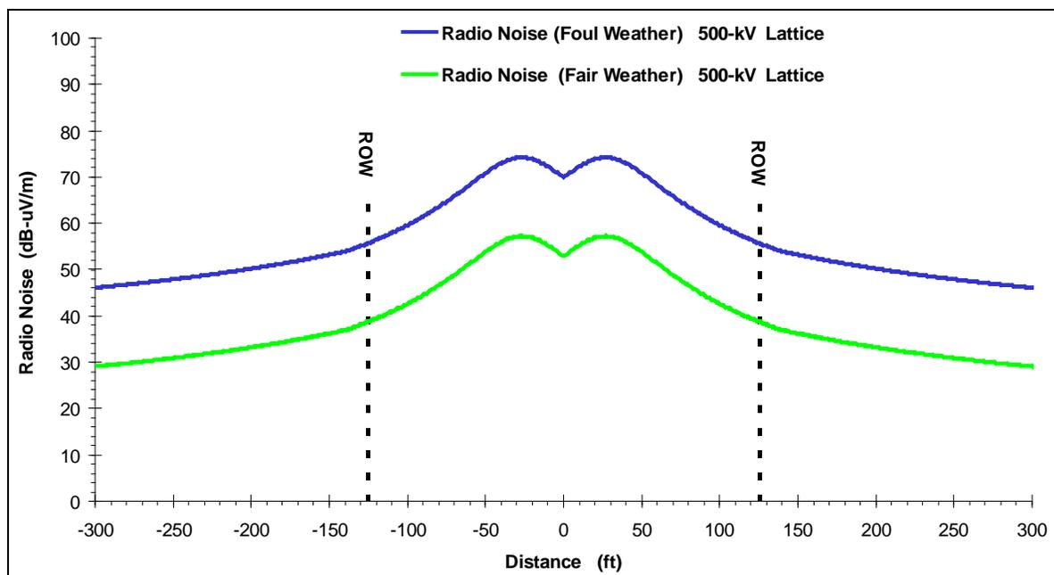
**Figure 3.21-16.** Radio Noise Profile at Midspan for Single-Circuit 500-kV Lattice Structure
