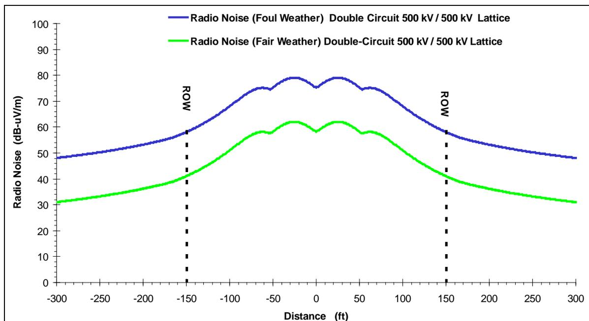
**Figure 3.21-17.** Radio Noise Profile at Midspan for Double-Circuit 500-kV Lattice Structure with Two 500-kV Circuits
