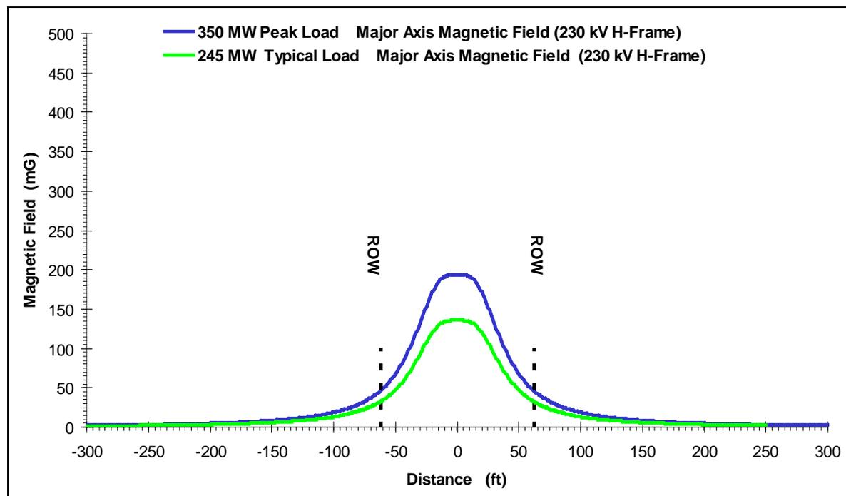
**Figure 3.21-7. Magnetic Field Profile at Midspan for 230-kV H-frame Structure**
