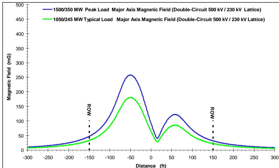
**Figure 3.21-10.** Magnetic Field Profile at Midspan for Double-Circuit 500-kV Lattice Structure with a 500-kV Circuit and a 230-kV Circuit
