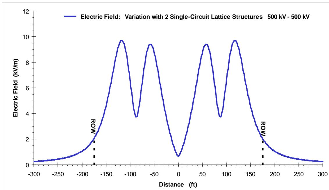
**Figure 3.21-20.** Electric Field Profile at Midspan for Two Single-Circuit 500-kV Lattice Tower Structures Both Energized at 500 kV (Segments 2, 3, and 4 under final energization plan)
