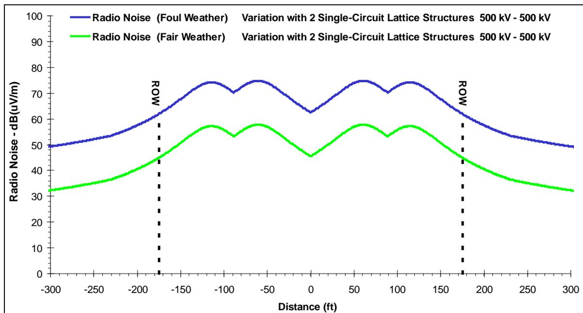
**Figure 3.21-26.** Radio Noise Profile at Midspan for Two Single-Circuit 500-kV Lattice Structures both Energized at 500 kV
