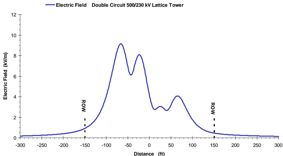
**Figure 3.21-6.** Electric Field Profile at Midspan for Double-Circuit 500-kV Lattice Structure with a 500-kV Circuit and a 230-kV Circuit
