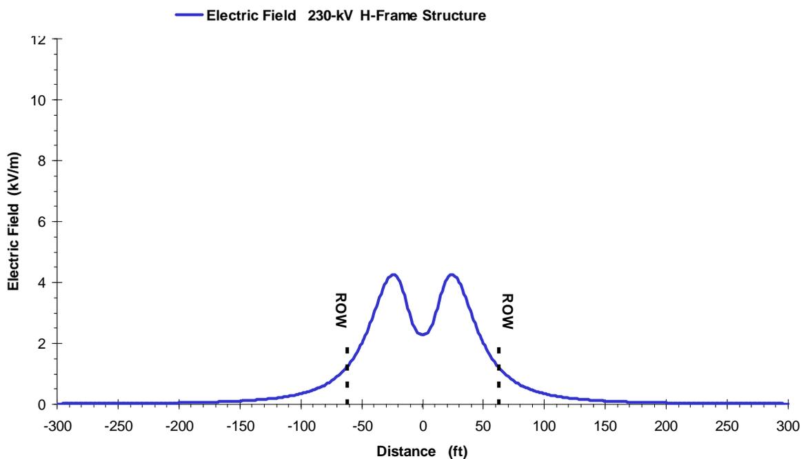
**Figure 3.21-3.** Electric Field Profile at Midspan for 230-kV H-frame Structure.
