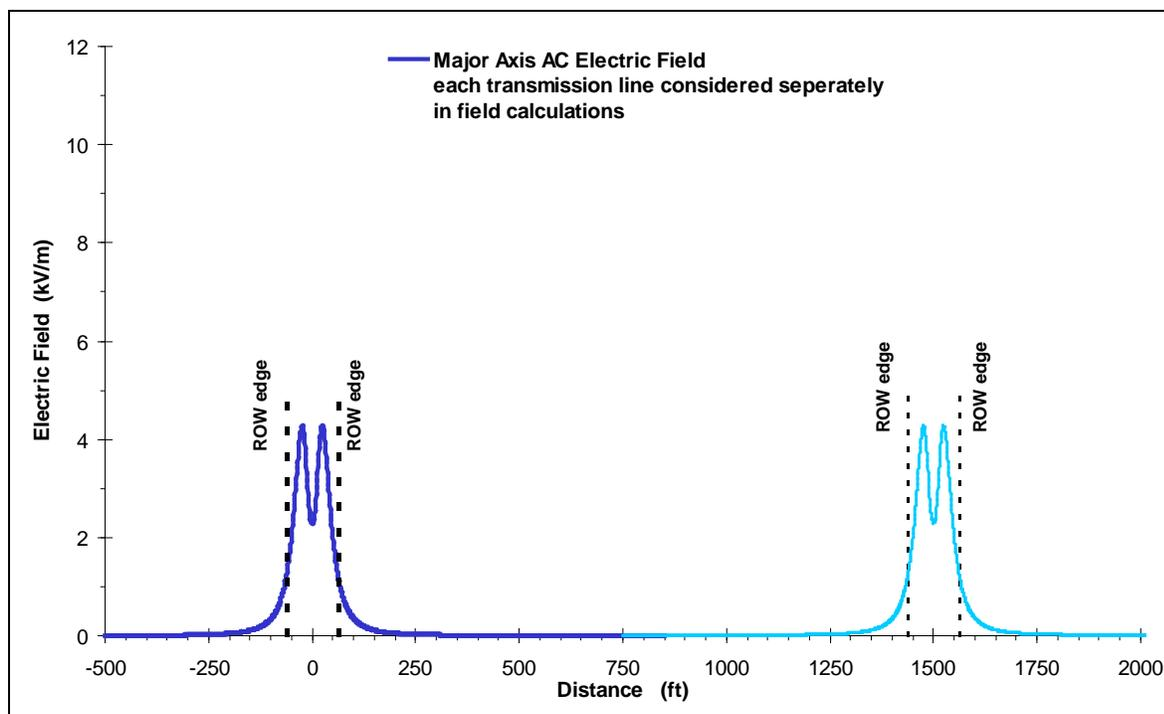
**Figure 3.21-2.** Plot of the Electric Field for Segment 1W Calculating the Electric Fields Separately for each of the Two Parallel Lines 1W(a) and 1W(c)
