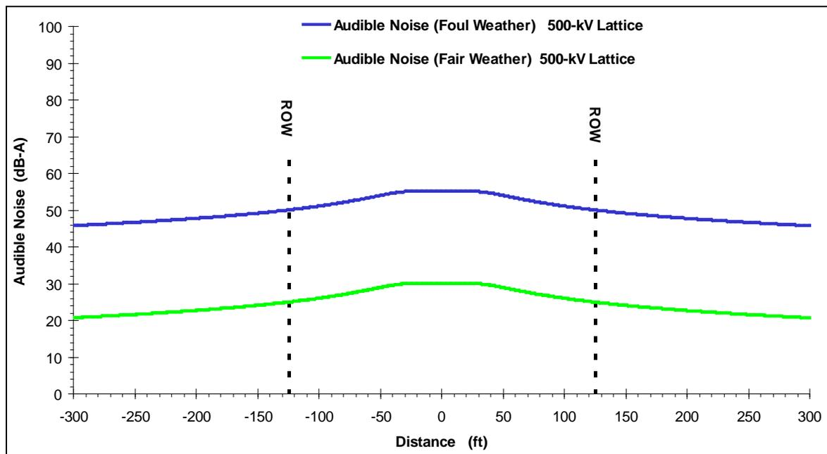
**Figure 3.21-12.** Audible Noise Profile at Midspan for Single-Circuit 500-kV Lattice Structure
