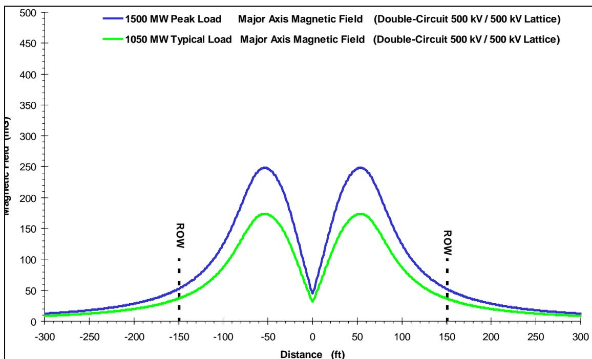
**Figure 3.21-9.** Magnetic Field Profile at Midspan for Double-Circuit 500-kV Lattice Structure with Two 500-kV Circuits
