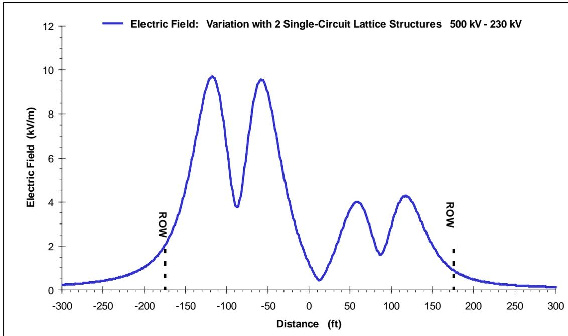
**Figure 3.21-21.** Electric Field Profile at Midspan for Two Single-Circuit 500-kV Lattice Tower Structures
