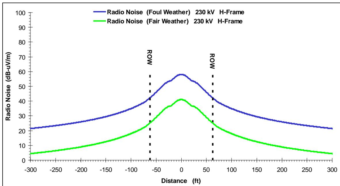
**Figure 3.21-15.** Radio Noise Profile at Midspan for Single-Circuit 230-kV H-frame Structure
