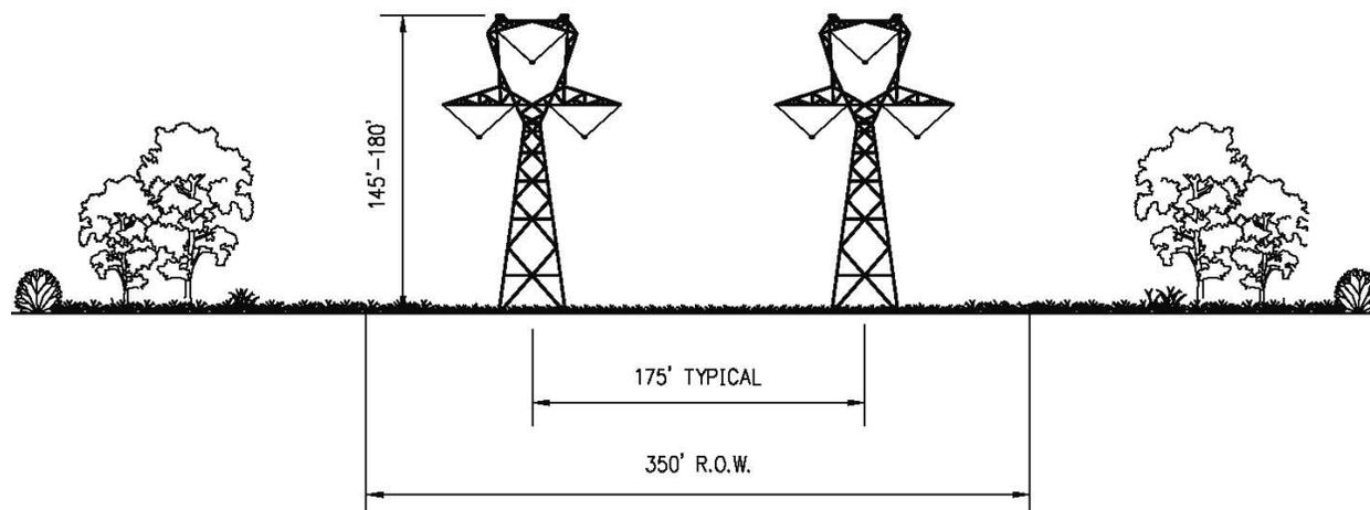
**Figure 3.21-19.** Proposed Design Variation for Two 500-kV Single Circuits
