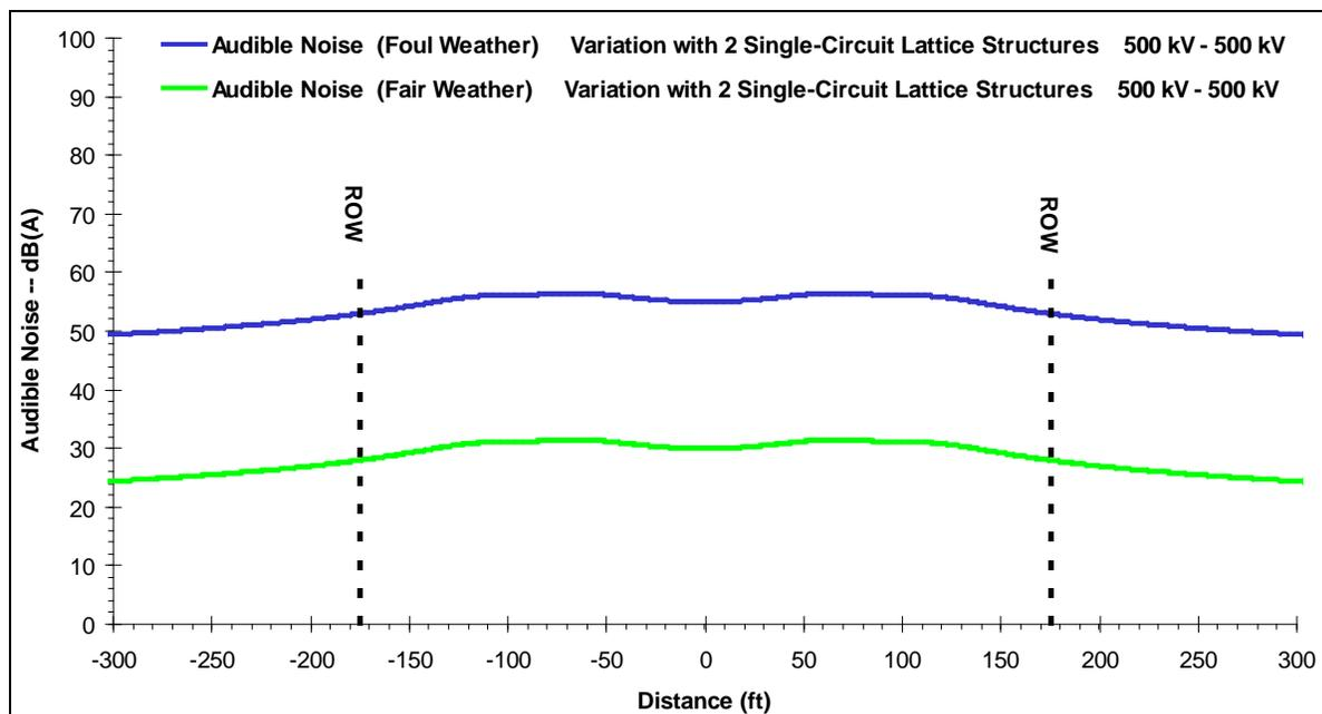
**Figure 3.21-24.** Audible Noise Profile at Midspan for two Single-Circuit 500-kV Lattice Structures
