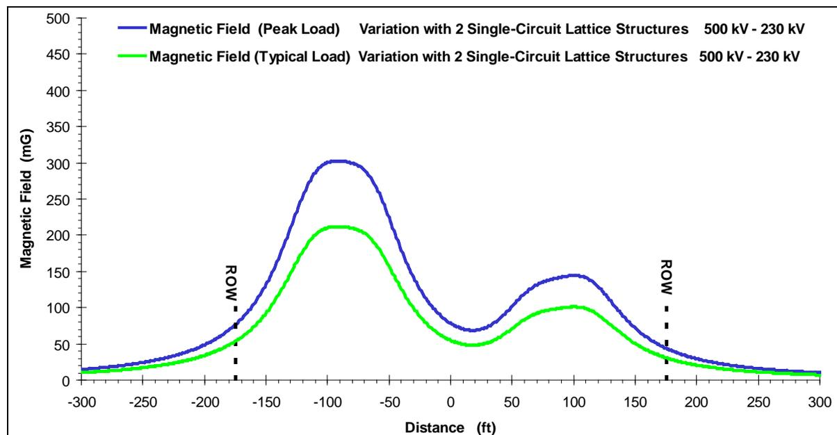
**Figure 3.21-23. Magnetic Field Profile at Midspan for Two Single-Circuit 500-kV Lattice Structures**
