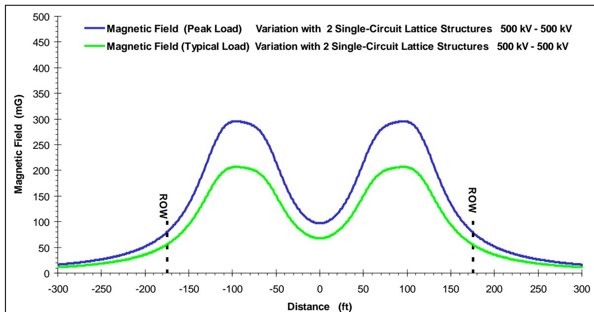
**Figure 3.21-22. Magnetic Field Profile at Midspan for Two Single-Circuit 500-kV Lattice Structures**
