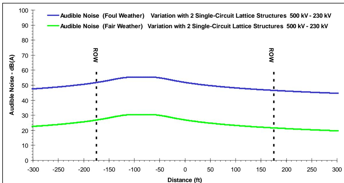
**Figure 3.21-25.** Audible Noise Profile at Midspan for two Single-Circuit 500-kV Lattice Structures
